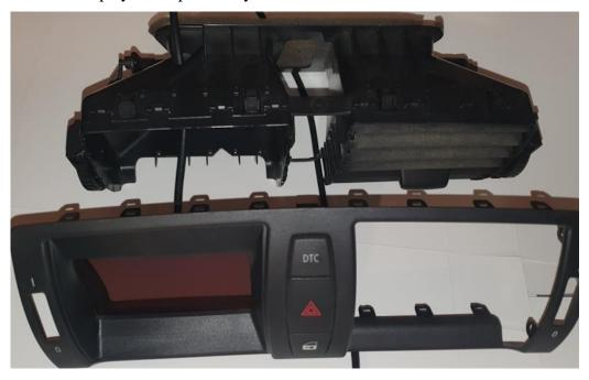
First place the cover with the display at the bottom because the cover must be tilted from bottom to top into the fresh air grill.
