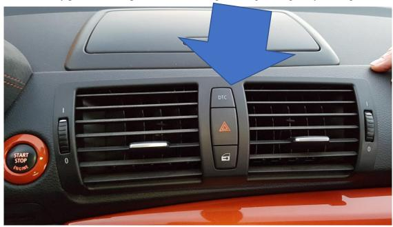
If the fresh air unit has been levered out at the top, pull it slightly forwards and upwards. Next, the plug for the switch unit must be removed:
