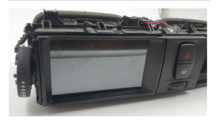
Put the fresh air grill incl. display back on the decorative strip. To do this, place the fresh air grill at the bottom and fold it up. Make sure that a bracket fits into the guides provided on each nozzle.
