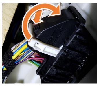
While the clip is folded down, the plug is pressed out of the FEM a bit and can then be removed.
