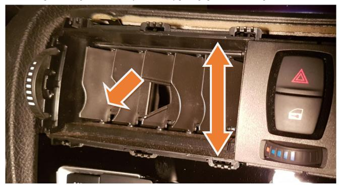
Drill a large enough hole for the display cable using the step drill provided:
