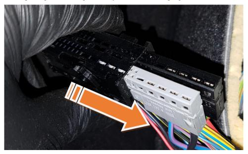
Now the cables Pin # 19 (CAN\_High with the color red / blue) and Pin 18 (CAN\_Low with the color red) are spun out. Use a small flat-head screwdriver, a needle or something similar. The crimp contacts have a flag which works like a barb. This flag must be pressed and at the same time carefully pulled on the cable.
