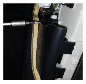
Insert the cover with the 3 plastic pins over the FEM and press firmly.
