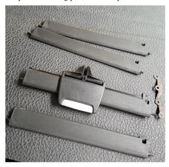
Pull off the connecting piece that may still be on the air ducts towards the driver's side or pull it out of the fresh air grille, this will later be attached to the display.
