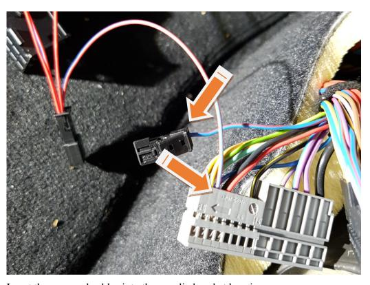
Insert the removed cables into the supplied socket housings.
