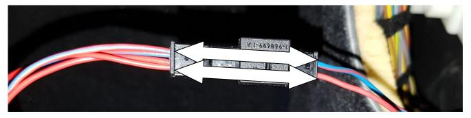
If both cables have been inserted into the socket housing, press the safety clip until it clicks into place. This again prevents slipping out of the contacts.
