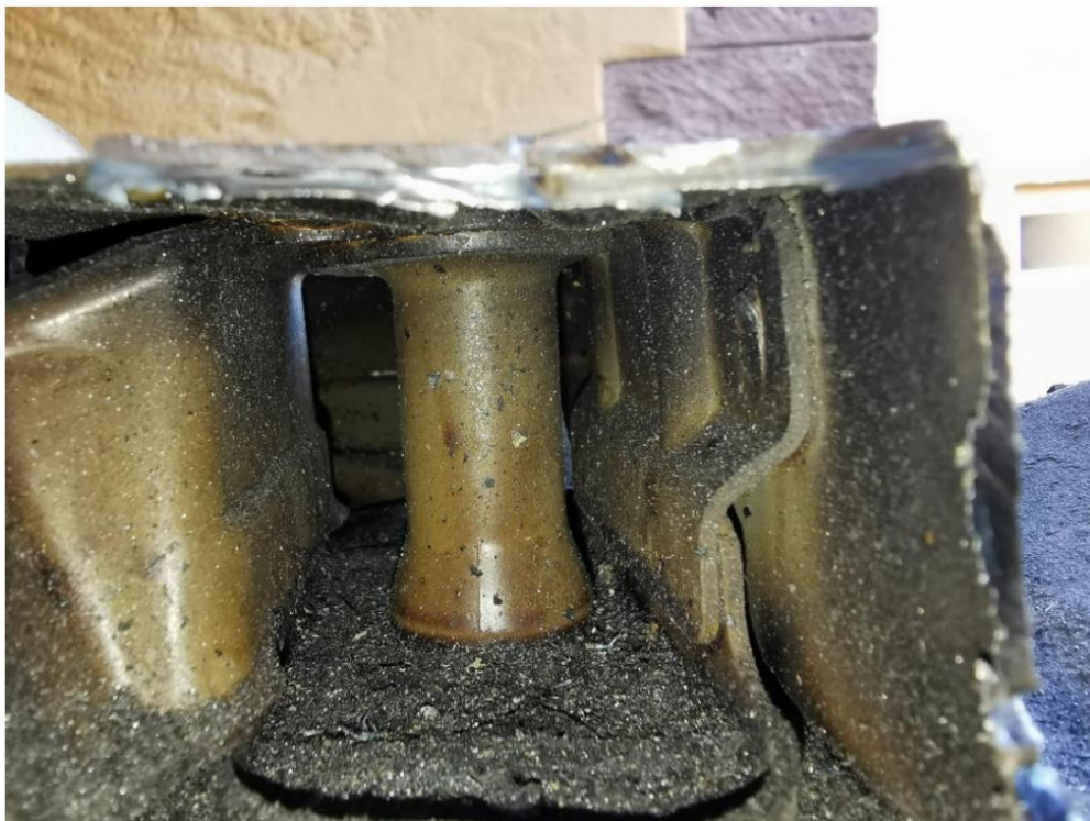
Picture below: inner spar, connection of the threaded sleeve (screwing point of the rear axle)
