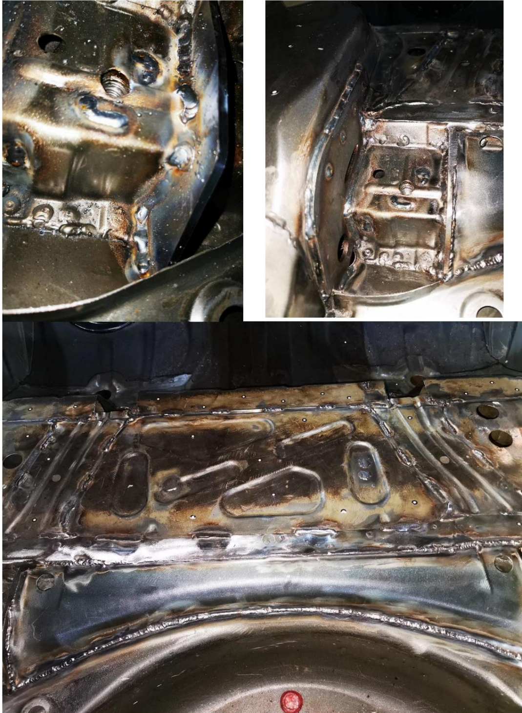
Image Top Left / Top Right: Close-ups before / after cleaning with the wire brush
