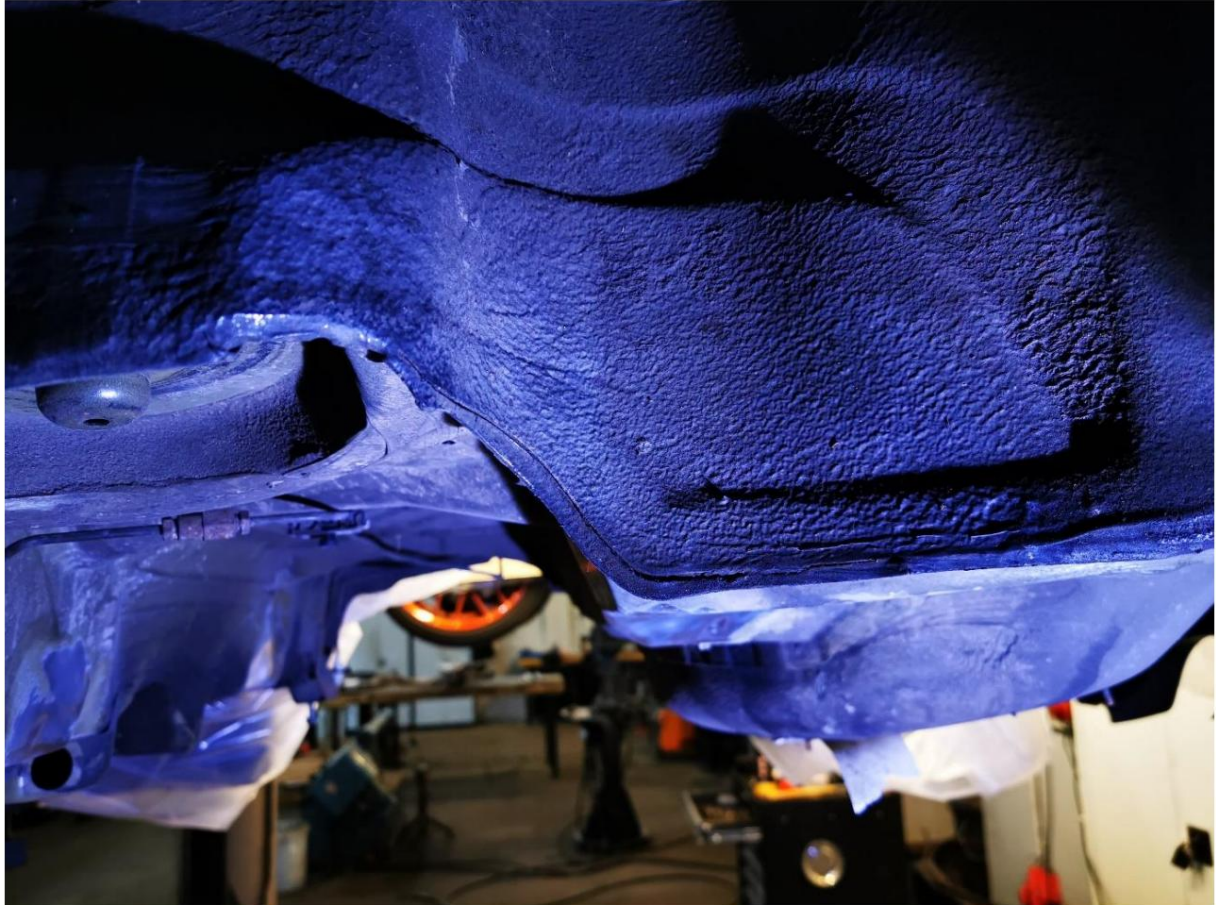
Picture above: Cracked spot welds between floor assembly and wheel arch, here Exceptionally visible despite underbody protection
