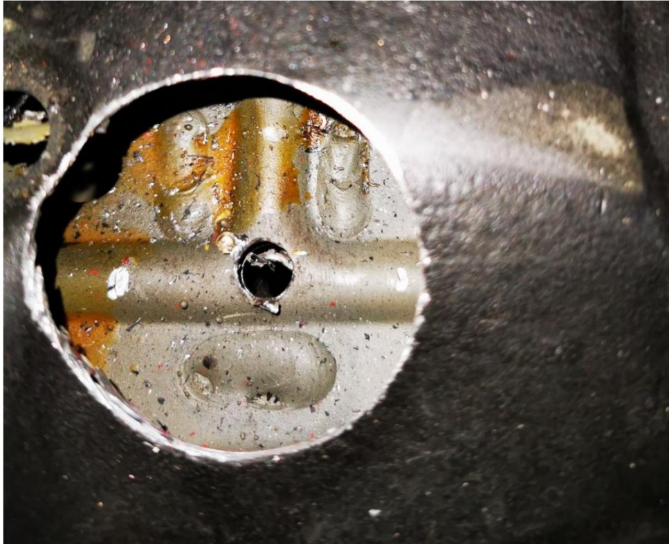
Picture above: Rear mounts after drilling with the visible embossing
