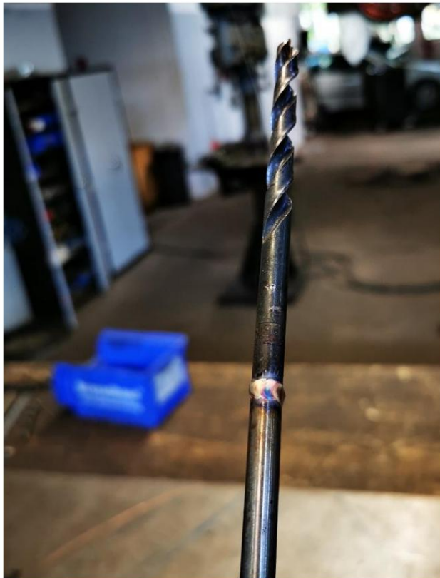
Image above: Extended drill bit with a long side cutting edge. Should be shortened to prevent the side cutting edges from damaging the threaded sleeve/thread of the chuck. Alternatively, use a drill bit with a smaller diameter.
